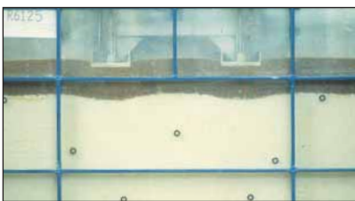
Figure 8: The University of Oxford, UK model footing experiments, without (top) and with (bottom) reinforcement at similar loads showing different behaviour.
