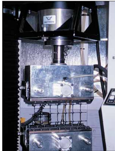
Figure 28: Test arrangement and result for ISO 10319 tensile test on Tensar SS30.
